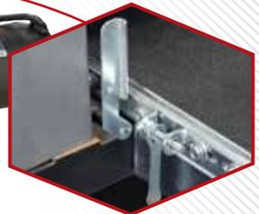
Fast Lever makes it easy to change alignment settings for narrow and wide stock.
